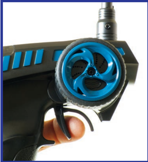
When at the mid position the model should remain stationary, if it creeps slightly adjust the throttle neutral dial accordingly.
