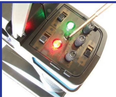
With the power on you can release the bind button once the green LED begins to flash to indicate the "Bind" process has initiated.
